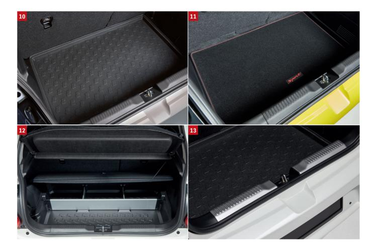
10 | CARGO TRAY1 <sup>1,2,3</sup> Waterproof with raised edges. Part No. 990E0-53R15-000
